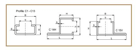
C 14H and C 15V steel profiles with punch hole in mounting rail
